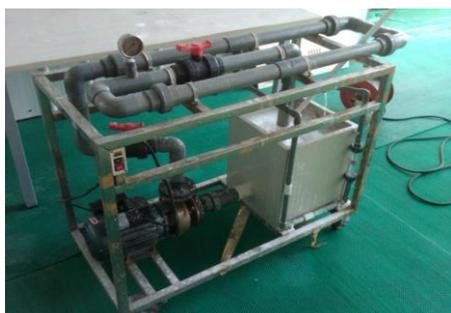
Figure 4 – Microfiltration Pilot Test Unit
