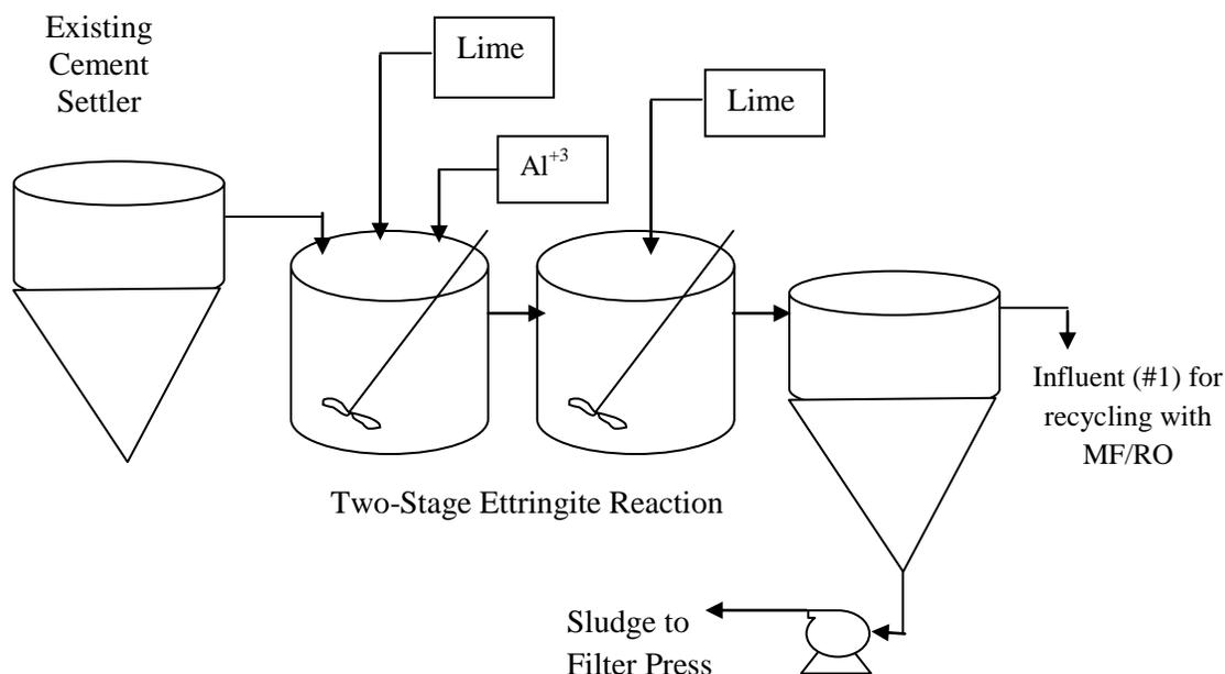
The sulfate depleted overflow from the settler will receive additional treatment for removal of residual sulfate and hardness by microfiltration before RO desalination. Approximately 88% of the raw wastewater will be recycled from the RO system to production for reuse, while the RO brine solution will be managed by one of the four options illustrated in Figure 7. These options are to be further justified based on the economic values.
