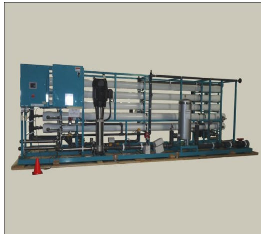
Figure: 6 Carbon Columns and RO Skids Prior to Installation
