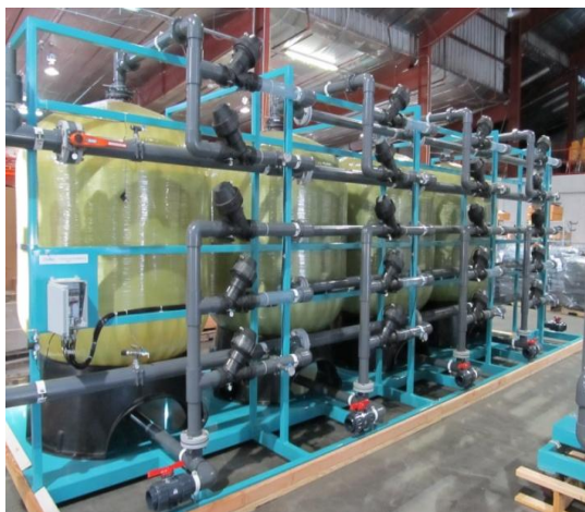
Figure: 6 Carbon Columns and RO Skids Prior to Installation
