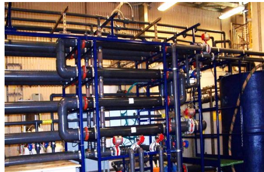
Figure 3 – Tubular MF Module Figure 4 – Tubular MF Skid (1 of 4 shown)
